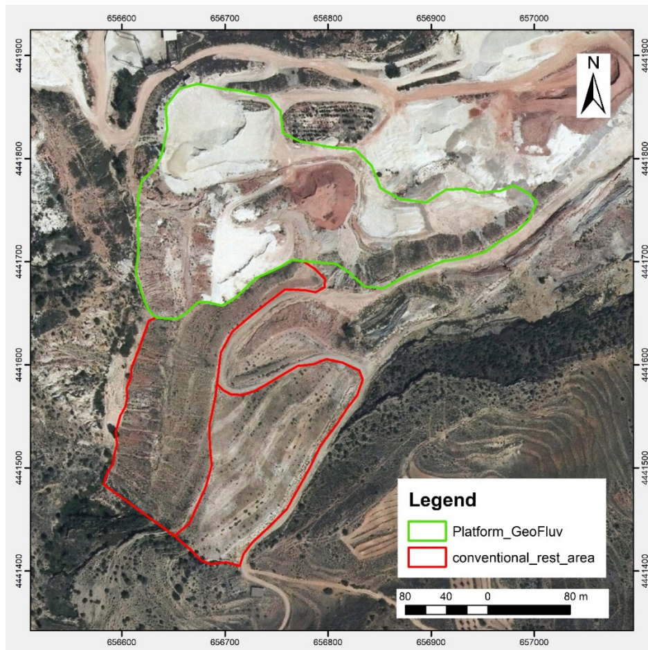
Figure 2. Fragment of the PNOA aerial orthophoto showing (approximately) the platform area that will be restored within the TECMINE project (green line) and the conventionally restored terraces where erosion has been measured (red line) (Coordinate System UTM-30N, Datum ETRS 1989).
