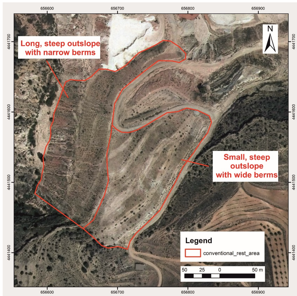
Figure 3. Fragment of the PNOA aerial orthophoto showing the two types of conventionally restored terraces, where erosion has been measured (Coordinate System UTM-30N, Datum ETRS 1989)
