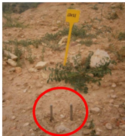
Figure 4. View of the pair of metal rods 20 cm deep into the soil to which the TDR is connected to measure moisture.
