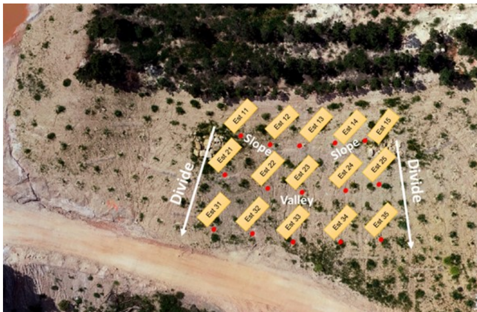
Figure 7. Distribution of sampling points in GeoFluv restoration with overburden substratum (GFEst) unit. The red dot corresponds to the sampling points and lines show the different landforms.
