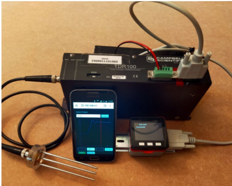
Figure 3. Campbell TDR 100 used to measure soil moisture content
