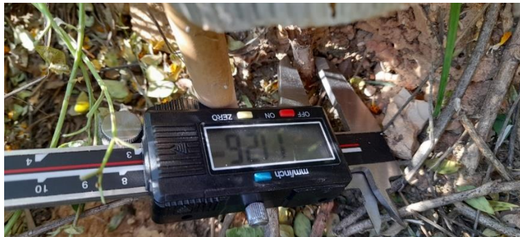
Figure 5. Detailed image of an electronic caliper measuring the stem basal diameter of a seedling.
