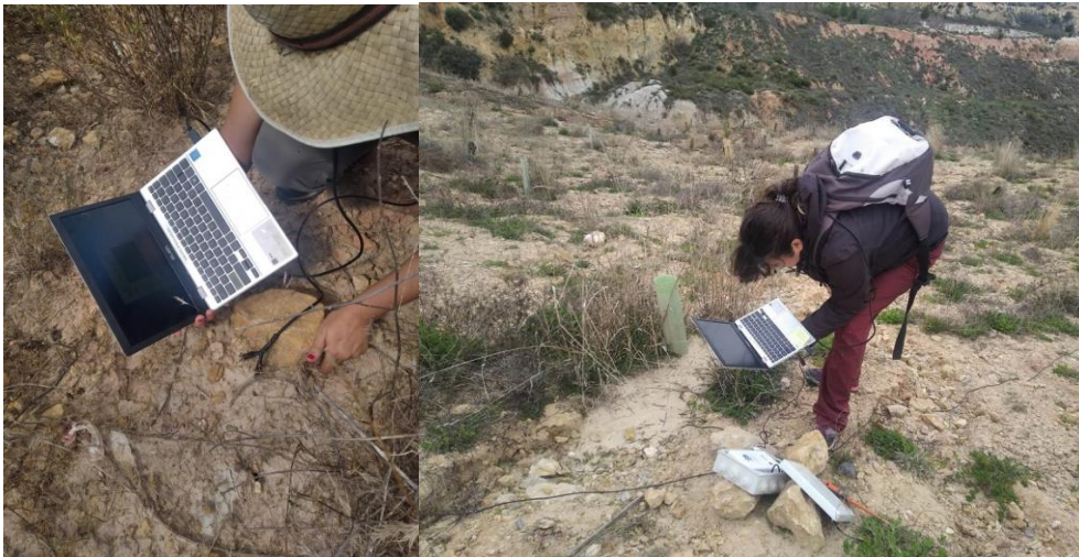
Figure 3. Detailed image of soil moisture samplings. Left image shows discrete measuring by the TDR100 Campbell device. Right image shows the downloading of continuous data through the software ECH20 Utility from Decagon.
