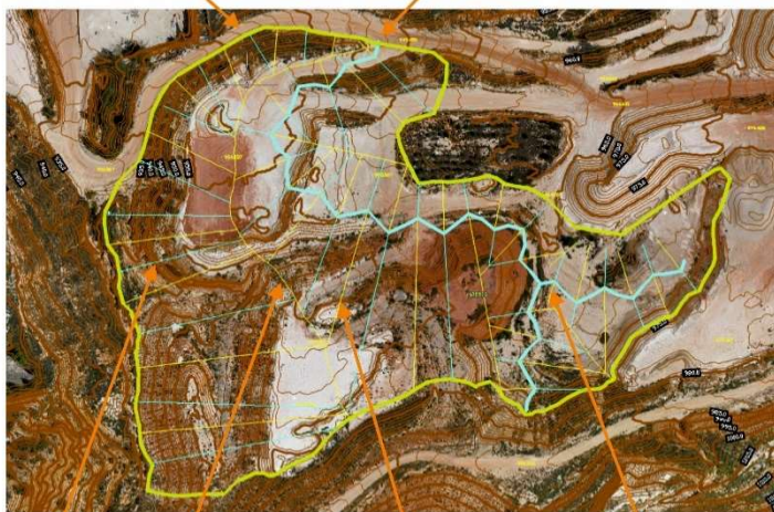
sub-channels (blue lines) main divide minor divides (yellow lines) fluvial channels to be built
