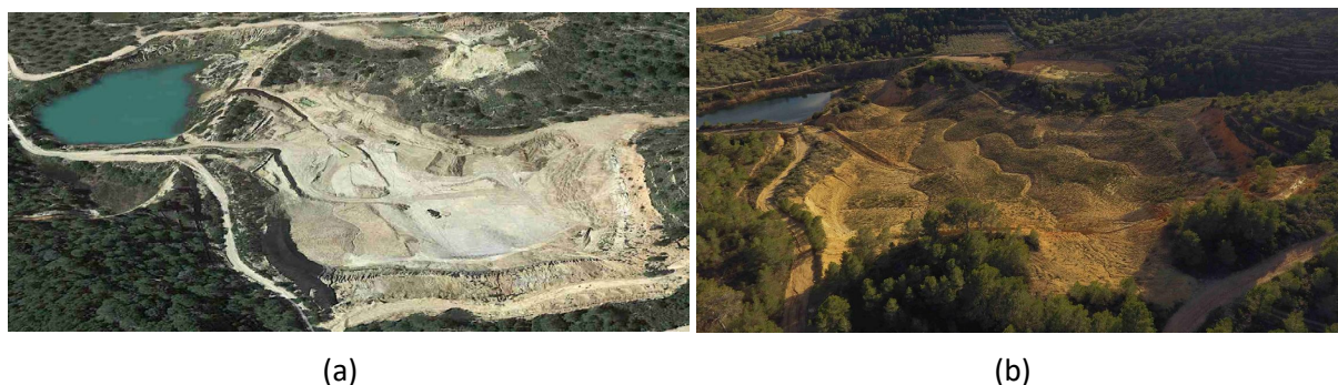
Figure 3 The Aurora geomorphic-based rehabilitation. (a) first advances of the geomorphic reconstruction (May 2015); (b) state in April 2018. LIFE ECOREST CLAY project. Photos by (a) Paisajes Españoles SA; (b) DIEDRO
