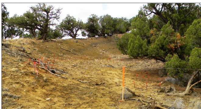
Fig. 11. N7 sediment dam site with survey in progress, horizontal string for full-pool elevation, and sediment pins installed.
