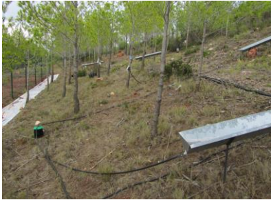
Gutters and tipping-bucket
