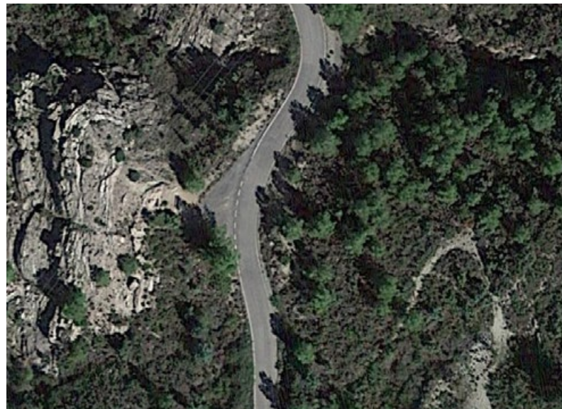
Figure 13. Passing places on roads with reduced width located at points with good visibility. Bejis-Arteas de Abaja section [Castellón]. Source: Google Maps.
